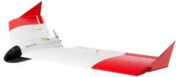
Figure 3. The Smartplanes SmartOne-C unmanned aircraft has a wingspan of 120 cm, a take-off weight of 1.2 kg (including camera) and a flight endurance of 45 minutes. The aircraft is hand launched and recovered by skid landing.
