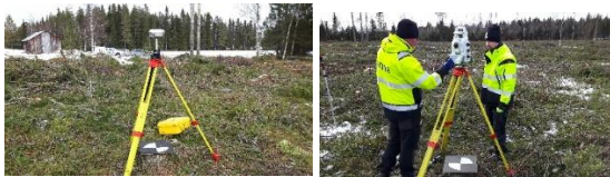
Figure 2 Static measurement of corner reference targets (left). Total station setup (right).
